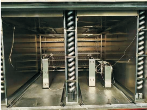
图1 试品在真空罐内的放置情况示意 Fig. 1 Schematic illustration of the placement of the test samples in the vacuum tank
